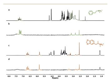
Fig. 8 (a)  $^1\text{H-NMR}$  spectrum of N-methylphenethylamine HCl (6, 2 mM), phenylalanine (14, 2 mM) and glucose (20 mM) in D $_2\text{O}$ . (b) NOE pumping-CPMGz spectrum of the same sample in the presence of S2-AuNP (3072 scans, 4 h). (c)  $^1\text{H-NMR}$  spectrum of a drug tablet dissolved in D $_2\text{O}$ . (d) NOE pumping-CPMGz spectrum of the same sample in the presence of S2-AuNP (3072 scans, 4 h). Conditions: [S2-AuNP] = 15  $\mu\text{M}$ , HEPES buffer 10 mM, and pD = 7.0.
