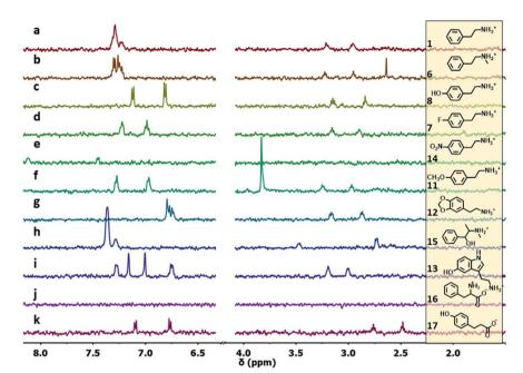
Fig. 4  $^{1}$ H-NMR NOE pumping-CPMGz sub-spectra (3072 scans, 4 h) of AuNP-S1 (14  $\mu$ M in D<sub>2</sub>O), HEPES buffer (10.0 mM) and different analytes (2 mM): (a)–(k). For 4-nitrophenethylamine (e), the NOE pumping spectrum is shown (same acquisition parameters). For 12 (g) and 15 (h), the signals respectively at 5.92, 5.11 and 1.04 ppm, present in the spectrum, are outside the spectral window shown for clarity (full spectra are reported in Fig. S23†).
