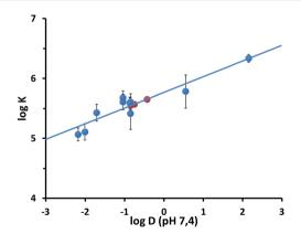
Fig. 5 Plot of the log K vs. log D (pH = 7.4) values relative to the binding of the luminescent analytes **8–13** and **17–19** to **S1**-AuNP. The lines represent the linear fit of the data (R = 0.885). Red circles report the affinity values estimated for substrates **1**, **14** and **15** on the basis of their log D values and the fitting parameters. The error bars reported represent the confidence intervals ( $3\sigma$ ) calculated from standard deviations reported in Table 1.
