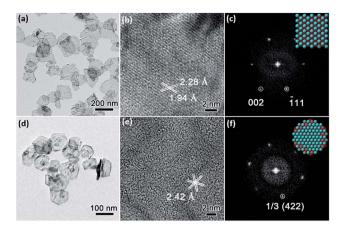
Fig. 3 Structural characterizations of (a–c) ultrathin PdNSs{110} and (d–f) PdNSs{111}. (a) TEM, (b) HRTEM images, and (c) corresponded FT pattern of PdNSs{110} synthesized using  $C_{22}$ –Py (Br<sup>-</sup>). (d) TEM, (e) HRTEM images, and (f) corresponded FT pattern of PdNSs{111} synthesized using  $C_{22}$ –QA (Cl<sup>-</sup>). The inset in (c) and (f) are schemes indicating the exposed surface facets.
