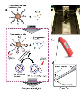
Scheme 1 (a) Schematic view of the design and working mechanism of the sensor based on a functional DNA and thermometer. (b) Photo of the photothermal chamber including a NIR laser pointer, and a 96-well colorless plate. (c) Photo of the super-fast Thermapen with 3 second readings that were used to detect the temperature change during laser irradiation. (d) Probe tip with a minimum immersion of 3.2 mm, which could measure the solution temperature in a small volume (180 µL).
