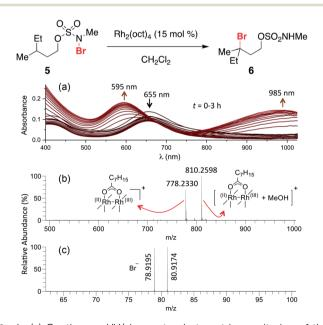
Fig. 1 (a) Continuous UV/vis spectrophotometric monitoring of the reaction of 5 shows an absorption spectrum characteristic of the conversion of a dinuclear  $\rm Rh^{2+}/Rh^{2+}$  complex ( $\lambda_{\rm max}=418$  nm and 655 nm) to a  $\rm Rh^{2+}/Rh^{3+}$  complex ( $\lambda_{\rm max}=595$  nm and 985 nm). High-resolution ESI-MS detected ion signals of (b)  $\rm Rh^{2+}/Rh^{3+}$  complex in positive ion mode, and (c)  $\rm Br^-$  in negative ion mode; see ESI† for experimental details.
