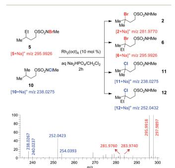
Fig. 2 High-resolution ESI-MS analysis shows that cross-halogenated products form in a competition experiment between bromosulfamate 5 and chlorosulfamate 10. Experimental m/z values (in the spectrum) agree well with the theoretical m/z values (underneath the chemical structures).
