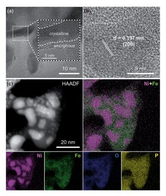
Fig. 2 (a) TEM image, (b) HRTEM image, (c) HAADF-STEM image and EDS elemental mapping images for the Ni<sub>2</sub>P@FePO<sub>x</sub> sample.
