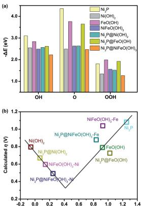
Fig. 6 (a) Calculated binding energies of the OER intermediates, and (b) volcano-shaped plot of calculated overpotential *versus* the differences in binding energies between OH and O on the simulated surfaces of different catalysts. NiFeO(OH) $_3$ -Ni and Ni $_2$ -P@NiFeO(OH) $_3$ -Ni represent the catalytic active sites for Ni, while NiFeO(OH) $_3$ -Fe and Ni $_2$ P@NiFeO(OH) $_3$ -Fe represent the catalytic active sites for Fe.
