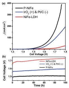
Fig. 7 (a) LSV curves of P-NiFe (black) and NiFe-LDH (red) as HER and OER bifunctional catalysts in 1.0 M KOH solution for overall water splitting. IrO $_2$  and Pt/C as OER and HER benchmarks were measured for comparison (blue). (b) Current density traces of CCE at 10 mA cm $^{-2}$  for overall water splitting in 1.0 M KOH for P-NiFe (black), NiFe-LDH (red), and commercial benchmarks of IrO $_2$  and 20% Pt/C (blue).
