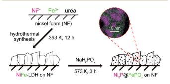
Scheme 1 The procedure for the synthesis of  ${\rm Ni_2P@FePO}_{\rm X}$  nanosheets.
