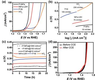
Fig. 5 (a) IR-corrected LSV curves, with a scan rate of 5 mV s $^{-1}$ . (b) Tafel plots for OER in 1.0 M KOH and (c) current density traces of CCE at 10 mA cm $^{-2}$  (as well as 100 and 1000 mA cm $^{-2}$  for P-NiFe, dashed line). (d) LSV curves of P-NiFe before (black square) and after (red circle) CCE for OER at 10 mA cm $^{-2}$  for 25 h. Catalysts: P-NiFe (black), NiFe-LDH (red), P-Ni (blue) and IrO<sub>2</sub> (orange).
