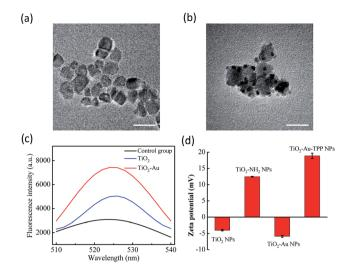
Fig. 1 Characterization of the nanoradiosensitizers. HRTEM images of the (a)  $TiO_2$  NPs and (b)  $TiO_2$ –Au NPs; the scale bars are 20 nm. (c) Fluorescence spectra of DBZTC (excitation = 490 nm, emission = 525 nm) after irradiation with X-rays. (d) Zeta potentials of each step of the modification:  $TiO_2$  NPs;  $TiO_2$ –NH $_2$  NPs;  $TiO_2$ –Au NPs; and  $TiO_2$ –Au–TPP NPs.
