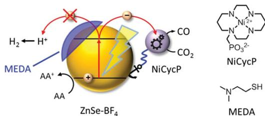
Fig. 1 Schematic representation of the photocatalyst system developed in this work: ligand-free ZnSe QDs ( $\text{ZnSe-BF}_4$ ) combined with a molecular electrocatalyst, NiCycP, for aqueous  $\text{CO}_2$  reduction to CO.  $\text{H}_2$  evolution can be partially suppressed by a surface inhibitor (MEDA). AA: ascorbic acid.
