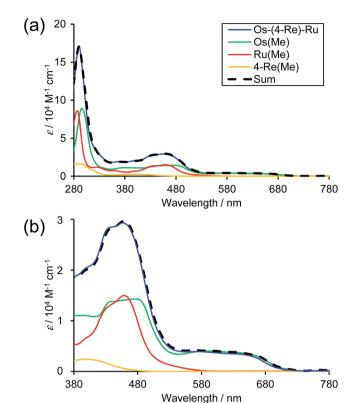
Fig. 3 UV-Vis absorption spectra of the obtained trinuclear complex (a) Os-(4-Re)-Ru (blue) and the corresponding mononuclear complexes, i.e. Os(Me) (green), Re(Me) (yellow) and Ru(Me) (red). The 1:1:1 summation spectrum of Os(Me), 4-Re(Me) and Ru(Me) is illustrated as a dotted line. The solvent was MeCN. (b) Enlarged spectra at  $\lambda_{abs} = 380$  to 780 nm.
