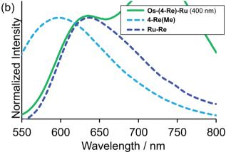
Fig. 4 (a) Emission spectra of Os–(4-Re)–Ru under irradiation at  $\lambda_{\rm ex}=400$  nm, 450 nm and 500 nm. The solvent was MeCN. (b) Enlarged emission spectrum of Os–(4-Re)–Ru at  $\lambda_{\rm ex}=400$  nm, which is mainly absorbed by the Re unit, with the emission spectra of 4-Re(Me) and Ru–Re.
