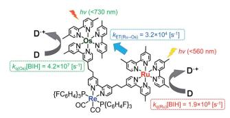
Fig. 11 Rate constants for the intramolecular energy transfer and reductive quenching by BIH.
