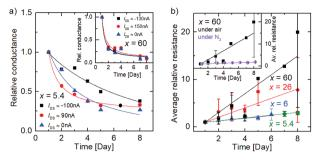
Fig. 3 Time dependent aging of the FGSs (a) relative conductance vs. time for FGSs with C/O ratios of x = 5.4 and x = 60 (inset) (b) average relative resistance for different values x as a function of time under air. The inset compares data where the sample (x = 60) was stored in air or under nitrogen atmosphere, respectively, for the whole time.
