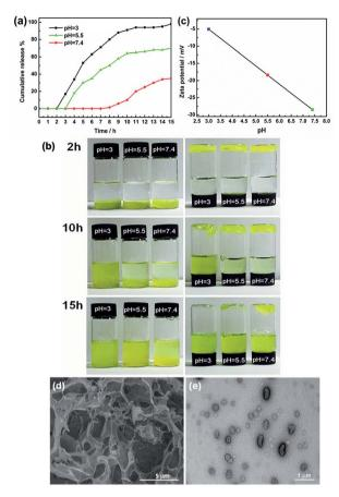
Fig. 7 (a) Release curves of Cur from AGC $_{16}$ /NTS gel at different pH. (b) Images of Cur release from AGC $_{16}$ /NTS gel at different pH. (c) Zeta potential of SO $_3$ <sup>-</sup> of NTS as a function of pH. (d) Cryo-SEM image of AGC $_{16}$ /NTS after drug release under pH 5.5 at 5 h. (e) TEM image of Cur-aggregates under pH 5.5 at 15 h.
