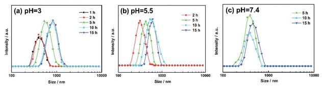
Fig. 8 Size changes of Cur-aggregations released from Cur-loaded hydrogels at pH 3 (a), 5.5 (b) and 7.4 (c).
