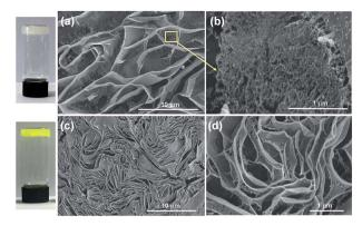
Fig. 4 Cryo-SEM images of (a and b) AGC  $_{\!16}/\!$  NTS and (c and d) Curloaded AGC  $_{\!16}/\!$  NTS hydrogel.
