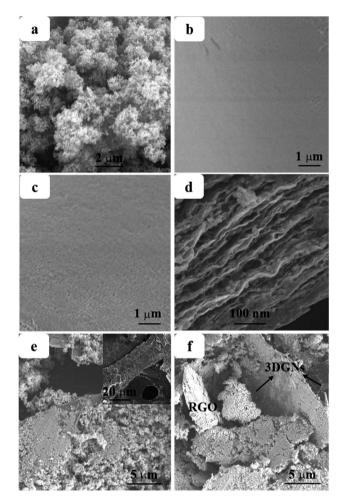
Fig. 1 SEM images of (a) TiO<sub>2</sub> (b) transport layer with the RGO as the terminal layer (c) transport layer with the TiO2 as the terminal layer (d) cross-section view of the transport layer (e) the 3DGNs added work laver (the original 3DGNs shown in the inset) (f) the 3DGNs and RGO co-modified work layer.
