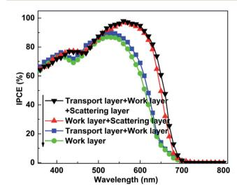
Fig. 8 IPCE patterns of devices with various photoanodes.
