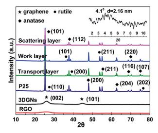
Fig. 2 XRD curves of the RGO, 3DGNs, TiO<sub>2</sub>, transport layer, work layer and scattering layer. The small angle XRD result of the transport layer is displayed as the inset.
