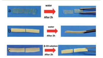
Fig. 10 Self-healing tests using different materials: (a) samples without CD-Al<sub>2</sub>O<sub>3</sub> NPs; (b) samples without PVP; (c) self-healing test of PVP/ p(HEMA-co-BA) after smearing cyclodextrin solution at cutting surface.
