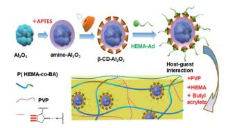
Fig. 1 Schematic of the process used in this study for the synthesis of self-healing material.
