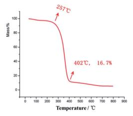
Fig. 8 Thermogravimetric curves of sample 3.
