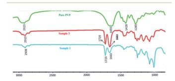
Fig. 5 Infrared spectrum of PVP and PVP/p(HEMA-co-BA) material.
