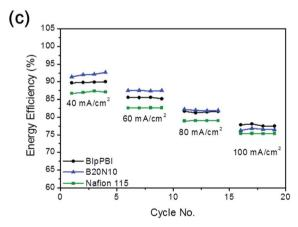
(a) CE, (b) VE, (c) EE of VRFB single cell performance test.
