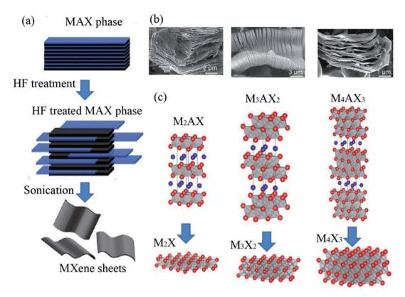
Fig. 1 (a) Early reported three different structures of MXenes (non-terminated):  $M_2X$ ,  $M_3X_2$  and  $M_4X_3$ . Reprinted from ref. 22 and 23 with permission. (b) SEM images of Ti<sub>2</sub>AlC, Ti<sub>3</sub>AlC<sub>2</sub> and Ta<sub>4</sub>AlC<sub>3</sub> after HF treatment (from right to left). (c) Schematic illustration of the synthesis of MXenes from MAX phases. Copyright 2013 John Wiley and Sons and Copyright 2012 American Chemical Society.
