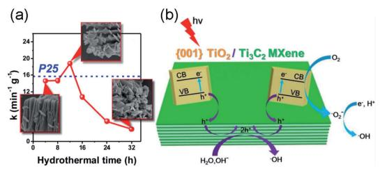
Fig. 4 (a) Photocatalytic degradation rate constant (k) of (001)TiO<sub>2</sub>/Ti<sub>3</sub>C<sub>2</sub> prepared for different hydrothermal times. (b) Schematic illustration of the charge-transfer process over (001)TiO<sub>2</sub>/Ti<sub>3</sub>C<sub>2</sub>. Reprinted from ref. 56 with permission. Copyright 2016 American Chemical Society.
