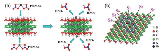
Fig. 3 (a) Schematic illustration of the formation of the  $Ti_3C_2(O_2H_{2-2m}Pb_m)$  structure from  $Ti_3C_2(O_1)_2$  to  $Ti_3C_2(O_2H_{2-2m}Pb_m)$ ; (b) top-view of the  $Ti_3C_2(O_2H_{2-2m}Pb_m)$  structure when the Pb coverage is 1/9 ML. S1–S6 represent the different atom sites of the hydroxyl. Reprinted from ref. 44 with permission. Copyright 2015 American Chemical Society.
