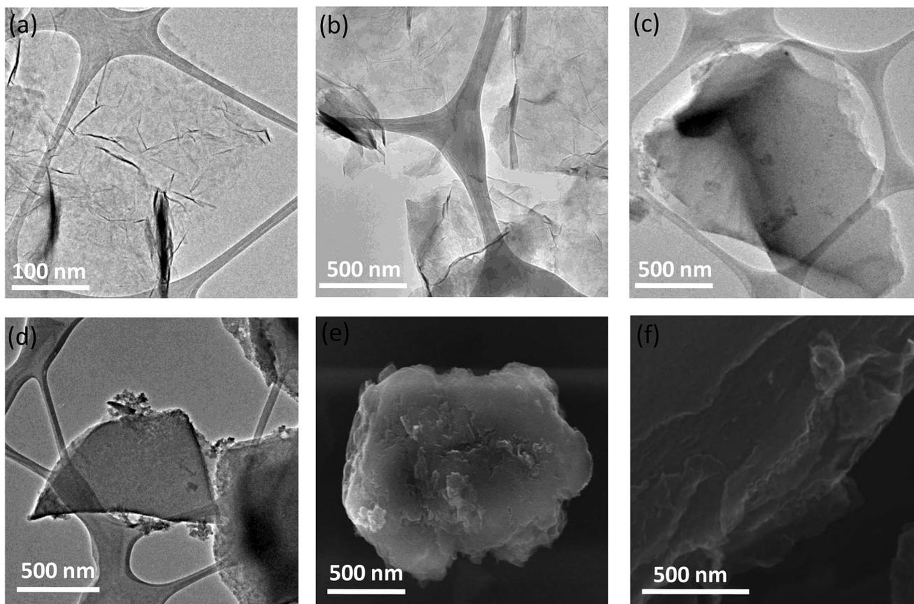
**Fig. 6** (a and b) HRTEM image of  $(\text{BN})_{0.3}\text{C}_{0.7}$ , (c and d) TEM image of BCN with cross-linking of graphene-graphene domains ( $\text{GG}/(\text{BN})_{0.3}\text{C}_{0.7}-(\text{BN})_{0.3}\text{C}_{0.7}$ ), (e) SEM image of  $\text{GG}/(\text{BN})_{0.3}\text{C}_{0.7}-(\text{BN})_{0.3}\text{C}_{0.7}$ , (f) BCN with cross-linking of graphene-BN/(BN) domains ( $\text{GBN}/\text{GG})_{0.3}\text{C}_{0.7}-(\text{BN})_{0.3}\text{C}_{0.7}$ ).
