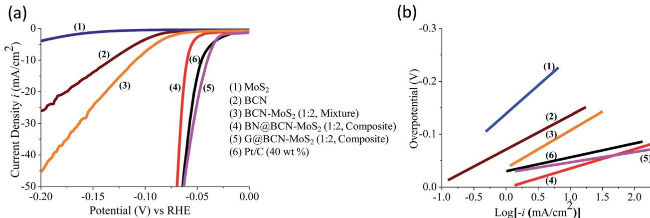
Fig. 21 HER electrocatalytic performance comparison. (a and b) Linear sweep voltammogram polarization curves and Tafel plots of (1) MoS<sub>2</sub>, (2) BCN, (3) BCN-MoS<sub>2</sub> (1 : 2, mixture), (4) BN/BCN-MoS<sub>2</sub> (1 : 2, composite) (5) G/BCN-MoS<sub>2</sub> (1 : 2, composite) samples including (6) Pt/C (40 wt%).
