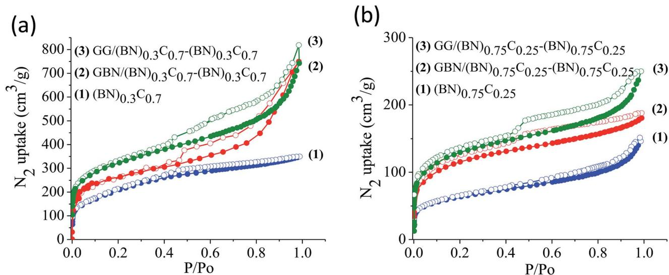
Fig. 9 Nitrogen sorption profiles of (a)  $(\text{BN})_{0.3}\text{C}_{0.7}$  (1),  $\text{GBN}/(\text{BN})_{0.3}\text{C}_{0.7}-(\text{BN})_{0.3}\text{C}_{0.7}$  (2),  $\text{GG}/(\text{BN})_{0.3}\text{C}_{0.7}-(\text{BN})_{0.3}\text{C}_{0.7}$  (3); (b)  $(\text{BN})_{0.75}\text{C}_{0.25}$  (1),  $\text{GBN}/(\text{BN})_{0.75}\text{C}_{0.25}-(\text{BN})_{0.75}\text{C}_{0.25}$  (2),  $\text{GG}/(\text{BN})_{0.75}\text{C}_{0.25}-(\text{BN})_{0.75}\text{C}_{0.25}$  (3) at 77 K.
