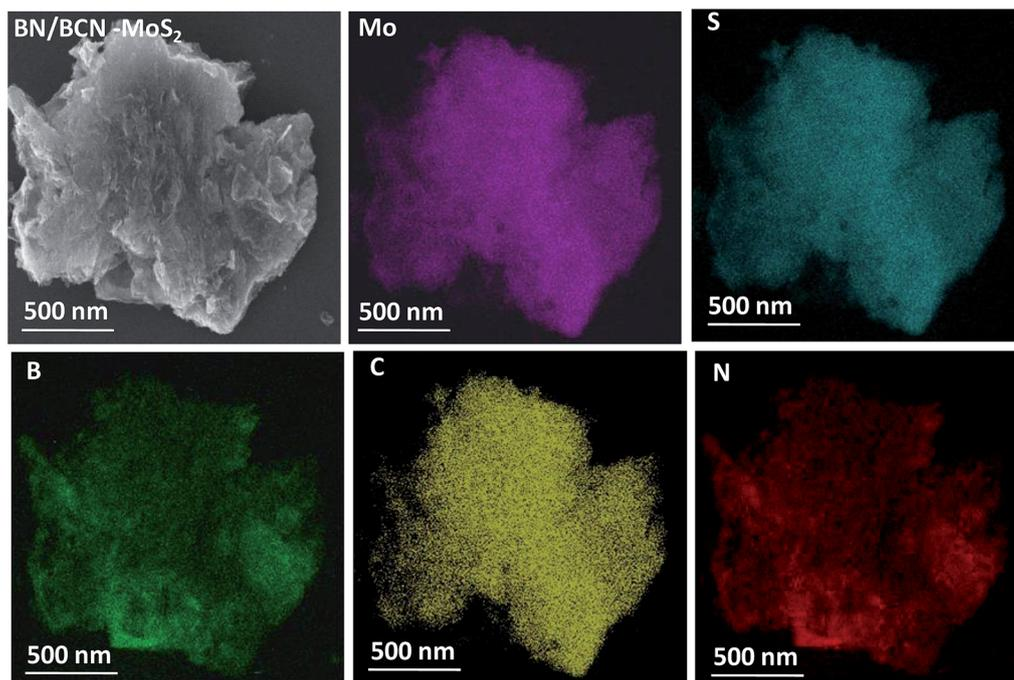
Fig. 14 Elemental mapping images of BN/BCN–MoS<sub>2</sub> nanocomposites (Mo, magenta; S, dark cyan; B, green; C, yellow; N, red) and FESEM image is given in top left corner.
