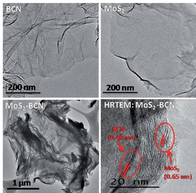
Fig. 15 TEM and HRTEM images of BCN, MoS<sub>2</sub> and MoS<sub>2</sub>–BCN nanocomposite.
