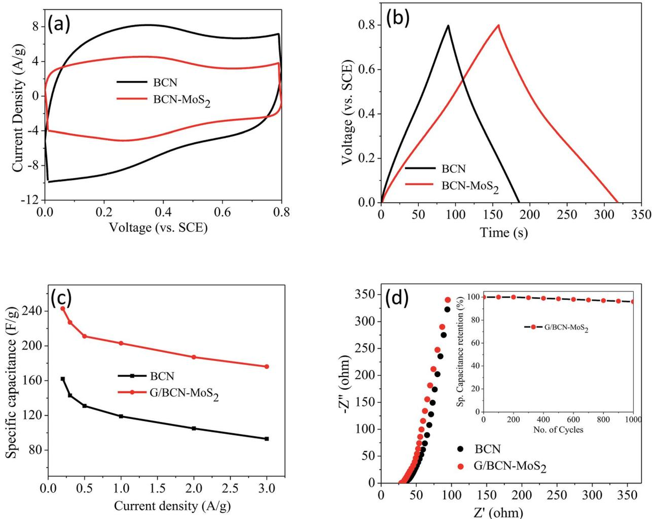
Fig. 20 (a) Cyclic voltammograms of BCN and G/BCN-MoS<sub>2</sub>, (b) Galvanostatic charge-discharge curves of BCN and G/BCN-MoS<sub>2</sub> at a current density of 1 A g<sup>-1</sup>, (c) specific capacitance vs. current density curves of BCN and G/BCN-MoS<sub>2</sub>, (d) Nyquist plots of BCN and G/BCN-MoS<sub>2</sub>.
