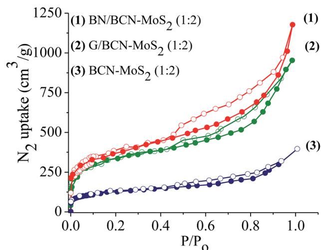
Fig. 19 Nitrogen sorption profiles of (1) BN/BCN–MoS<sub>2</sub> (1 : 2), (2) G/BCN–MoS<sub>2</sub> (1 : 2) and (3) BCN–MoS<sub>2</sub> (1 : 2) mixture.
