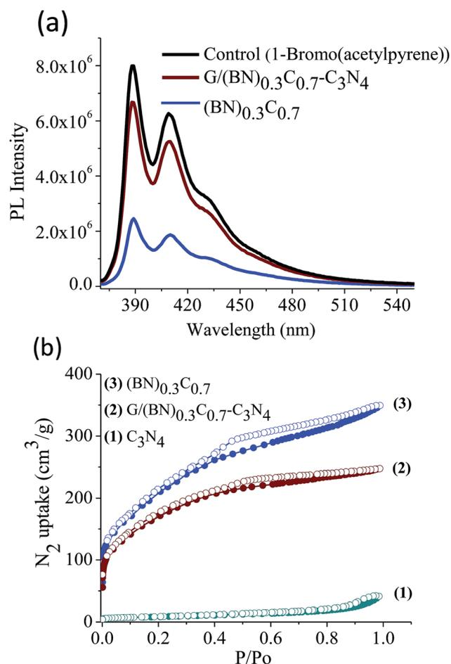
**Fig. 13** Emission spectra of 1-(bromoacetyl)pyrene reacted with carboxylic groups of (a)  $(\text{BN})_{0.3}\text{C}_{0.7}$  (blue),  $\text{G}/(\text{BN})_{0.3}\text{C}_{0.7}$ – $\text{C}_3\text{N}_4$  (wine), with the control experiment; (b) nitrogen sorption profiles of  $(\text{BN})_{0.3}\text{C}_{0.7}$  (blue),  $\text{G}/(\text{BN})_{0.3}\text{C}_{0.7}$ – $\text{C}_3\text{N}_4$  (wine),  $\text{C}_3\text{N}_4$  (dark clay) at  $77 \text{ K}$ .
