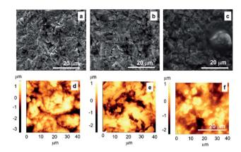
Fig. 5 SEM (a-c) and AFM (d-f) micrographs of the Gum alloy (a and d) functionalized with GNP (b and e), and GNP-SS (c and f) by MAPLE (266 nm, 600 mJ cm<sup>-2</sup>). The scanned area by AFM was  $40 \times 40 \, \mu m^2$ . Scale bar: 20 µm.
