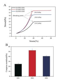
Fig. 4 (A) The stress-strain curves of SA/PEG hydrogels by a linear 1 N min<sup>-1</sup> ramp force loading to test the breakage strength. (B) The compressive modulus of the SA/PEG hydrogels.
