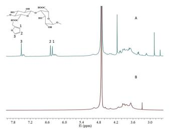
Fig. 1  $\,^{1}$ H-NMR spectra in D<sub>2</sub>O (400 MHz) of SA (B) and SA-furan (A) showing that the furan groups were successfully grafted to SA. The peaks at 6.26, 6.46 and 7.51 ppm (furan protons) are indicated by 1, 2 and 3
