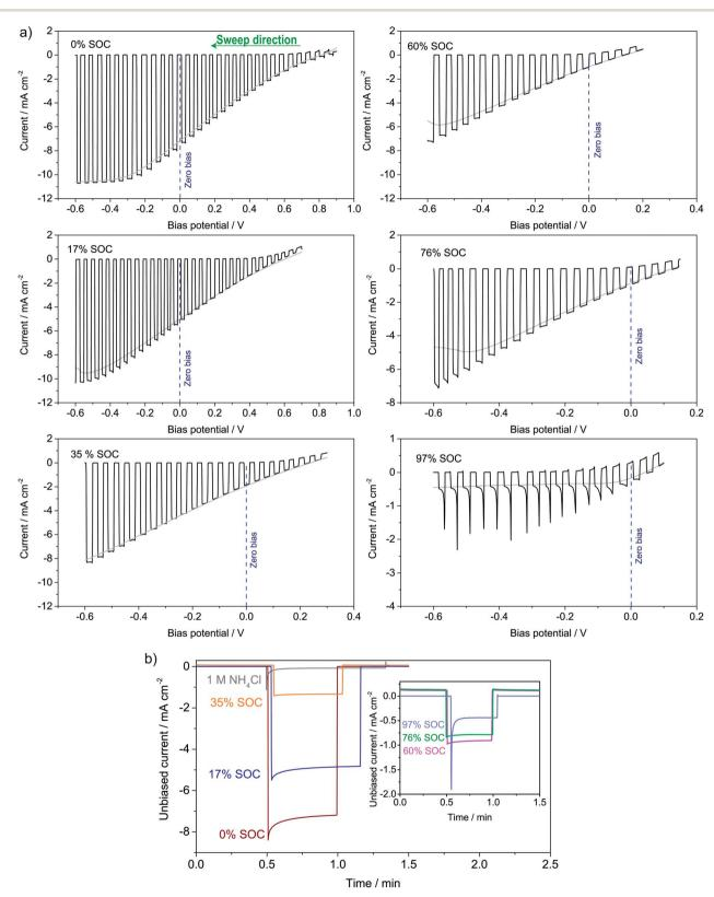
Fig. 6 (a) LSVs on pn $^+$ Si/TiO $_2$  recorded in the solar flow battery cell using the same concentration anolyte and catholyte as in the battery cycling tests. The electrolytes were brought to the indicated SOC in the RFB cell. (b) The unbiased photocurrent density at the same SOCs recorded as the light is turned on (at the time *ca.* 0.5 minute); the inset shows the higher SOCs.
