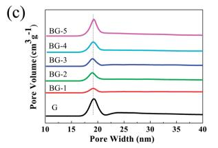
Fig. 3 (a) Nitrogen adsorption—desorption isotherms, (b) specific surface area column (column graph) and pore volume (line graph) and (c) pore size distribution plot.
