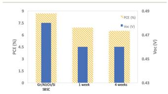
Fig. 7 Variation of PCE and  $V_{\rm oc}$  of Gr/Si with  ${\rm Al_2O_3}$  interfacial layer over time.
