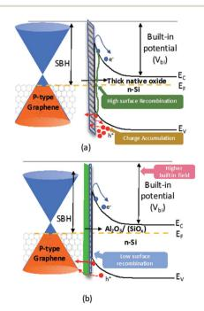
Fig. 6 Energy band diagrams of Gr/Si SBSC (a) with thick interfacial layer (b) with Al<sub>2</sub>O<sub>3</sub>/native oxide interfacial layers.
