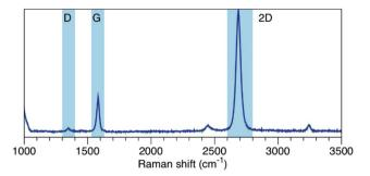
Fig. 1 Raman spectrum of synthesized graphene.28
