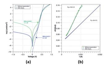
Fig. 5 (a) Dark J-V characteristics of Gr/Si solar cells with and without  $Al_2O_3$  interfacial layer. Inset shows the corresponding ln J-V curves. (b) Plots of dV/dln(I) versus I for Gr/Si solar cells with and without Al<sub>2</sub>O<sub>3</sub> interfacial layer.
