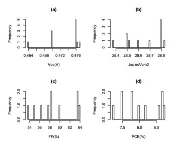
Fig. 4 Histogram of (a) open circuit voltage (b) short circuit current (c) fill factor (d) power conversion efficiency for Gr/Si solar cells with Al<sub>2</sub>O<sub>3</sub> interfacial layer.
