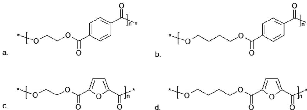
Fig. 10 Comparison of the polymer structures obtained from terephthalic and 2,5-furandicarboxylic acid:<sup>184</sup> (a) poly(ethylene terephthalate) PET; (b) poly(butylene terephthalate) PBT; (c) poly(ethylene 2,5-furandicarboxylate) PEF; (d) poly(butylene 2,5-furandicarboxylate) PBF.
