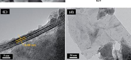
Fig. 2 (a) Cross-section SEM image of  $Ti_3C_2$  particles; (b) EDS spectrum of  $Ti_3C_2$  MXene, revealing the chemical composition of MXene; (c) cross-section TEM image of a 4-layer  $Ti_3C_2$  flake, the estimated inter-layer space is about 1 nm; (d) TEM image of a 2-layer  $Ti_3C_2$  flake.
