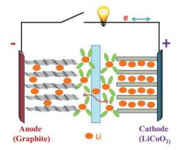
Fig. 1  $\,$  Schematic of a lithium-ion battery during the charge/discharge process. $^{25}$
