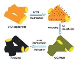
Fig. 14 Schematic of the fabrication of rGO enwrapped  $\mbox{V}_2\mbox{O}_5$  nanorods.  $^{140}$
