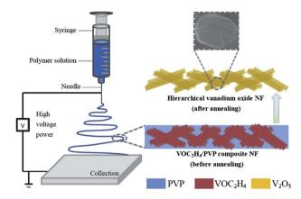
Fig. 6 Schematic showing the strategy for fabricating hierarchical  $V_2O_5$  nanofibers.<sup>79</sup>
