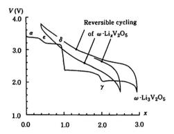
Fig. 2 Various phases associated with the electrochemical intercalation of lithium into  $\rm V_2O_5.^{40}$
