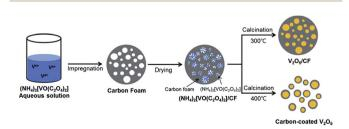
Fig. 12 Schematic of the preparation of carbon-fabricated V<sub>2</sub>O<sub>5</sub> samples (CF300 and CF400).117
