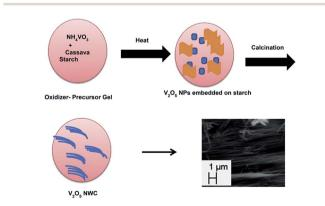
Fig. 4 Illustration of V<sub>2</sub>O<sub>5</sub> NWC formation.<sup>69</sup>
