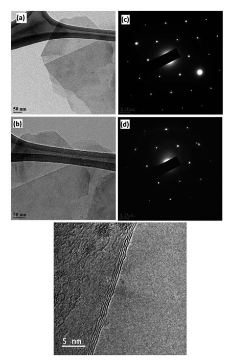
Fig. 2 TEM images [(a) and (b)] showing few layers of graphene and their corresponding diffraction patterns [c & d] showing six-membered rings. (e) HRTEM images showing few layers of graphene.
