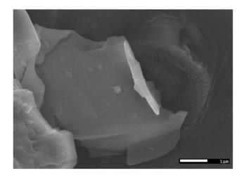
Fig. 3 FEG-SEM images showing the graphene flakes of  $\sim$ 3  $\mu m$ .
