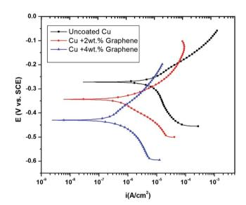
Fig. 6 Potentiodynamic polarization curves of Cu in 3.5 wt% NaCl after graphene coating showing lower corrosion current densities.
