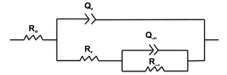
Fig. 9 Equivalent circuit used to simulate the EIS data.
