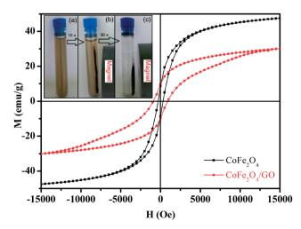
Fig. 6 Magnetization curves of CoFe<sub>2</sub>O<sub>4</sub> and CoFe<sub>2</sub>O<sub>4</sub>/GO. The inset shows the photographs of the separation processes of CoFe<sub>2</sub>O<sub>4</sub>/GO: (a) without external magnetic field, and (b, c) with external magnetic field.
