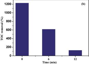
Fig. 7 UV-vis spectra of RhB solution at different times using  $CoFe_2O_4/GO$  as a catalyst (a); the TOC removal efficiency of RhB using  $CoFe_2O_4/GO$  as a catalyst.
