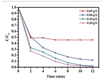
Fig. 10 Effect of oxone concentration on RhB degradation over  $CoFe_2O_4/GO$ . Reaction conditions: [RhB] = 0.03 mmol L<sup>-1</sup>, amount of catalyst = 10 mg, T = 25 °C.
