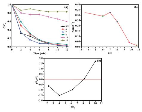
Fig. 13 Effect of pH on RhB degradation over the CoFe<sub>2</sub>O<sub>4</sub>/GO catalyst (a, b); point zero charge of CoFe<sub>2</sub>O<sub>4</sub>/GO. Reaction conditions: [RhB] = 0.03 mmol L<sup>-1</sup>, [PMS] = 0.10 mmol L<sup>-1</sup>, amount of catalyst = 10 mg, T = 25 °C.
