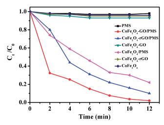
**Fig. 8** RhB degradation by various catalytic PMS systems. Conditions:  $[RhB]_0 = 0.03 \text{ mmol L}^{-1}$ ,  $[PMS] = 0.10 \text{ mg L}^{-1}$ , amount of catalyst = 10 mg, temperature = 25 °C.
