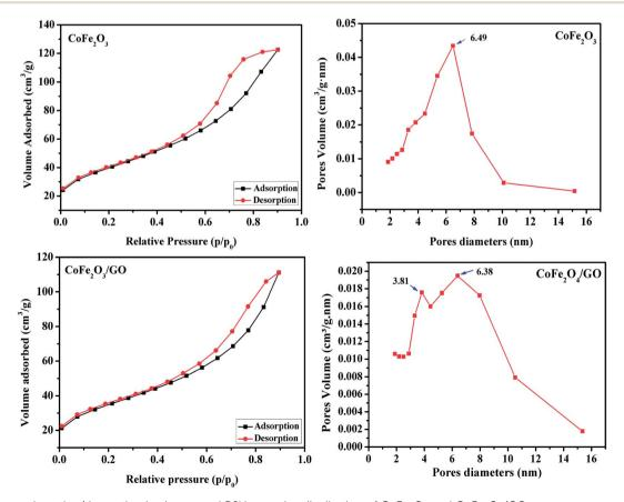
Nitrogen adsorption/desorption isotherms and BJH pore size distribution of CoFe<sub>2</sub>O<sub>4</sub> and CoFe<sub>2</sub>O<sub>4</sub>/GO.
