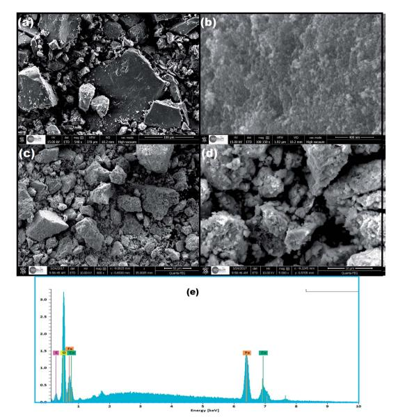
Fig. 4 SEM images of (a, b) CoFe<sub>2</sub>O<sub>4</sub> and (c, d) CoFe<sub>2</sub>O<sub>4</sub>/GO, (e) EDX of CoFe<sub>2</sub>O<sub>4</sub>/GO.
