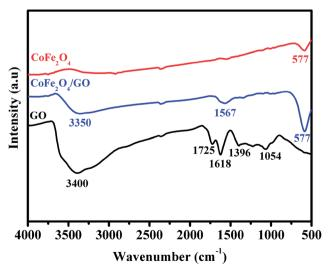
Fig. 2 FT-IR spectra of GO, CoFe<sub>2</sub>O<sub>4</sub> and CoFe<sub>2</sub>O<sub>4</sub>/GO.
