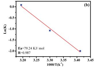
Fig. 11 The effect of reaction temperature on RhB degradation over the CoFe<sub>2</sub>O<sub>4</sub>/GO catalyst (a); the Arrhenius plot with linear regression (b); reaction conditions:  $[RhB] = 0.03 \text{ mmol L}^{-1}$ , amount of catalyst = 10 mg and  $0.1 \text{ g L}^{-1}$  of oxone at different temperatures.
