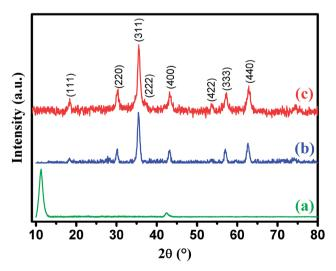
Fig. 1 XRD patterns of graphene oxide (a), CoFe<sub>2</sub>O<sub>4</sub> (b) and CoFe<sub>2</sub>O<sub>4</sub>/ GO (c).
