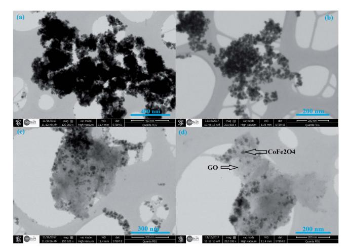
Fig. 5 STEM images of CoFe<sub>2</sub>O<sub>4</sub> (a, b) and CoFe<sub>2</sub>O<sub>4</sub>/GO (c, d)
