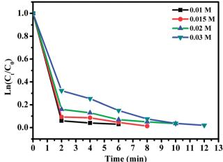
Fig. 12 Effect of RhB concentration. Reaction conditions: [PMS] =  $0.1 \text{ mmol L}^{-1}$ ; amount of catalyst = 10 mg,  $T = 25 \,^{\circ}\text{C}$ .
