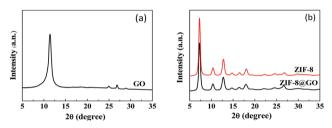
Fig. 2 XRD patterns recorded for (a) GO and (b) ZIF-8, ZIF-8@GO.
