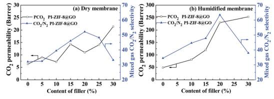
Fig. 12 Comparison of the mixed gas separation performance observed for the dry and humidified membranes: (a)  $CO_2$  permeability and  $CO_2/N_2$  selectivity observed for the dry membranes with the ZIF-8@GO based MMMs (1.0 bar, 30 °C).
