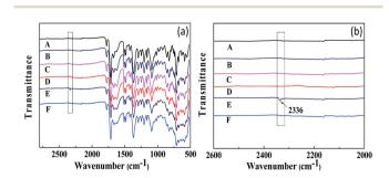
Fig. 11 FT-IR spectra of  $CO_2$  adsorption and desorption within the humidified membranes. (A) PI membrane; (B)  $CO_2$ -absorbed PI membrane; (C)  $CO_2$ -desorbed PI membrane; (D) PI-ZIF-8@GO-20 membrane; (E)  $CO_2$ -absorbed PI-ZIF-8@GO-20 membrane; (F)  $CO_2$ -desorbed PI-ZIF-8@GO-20.
