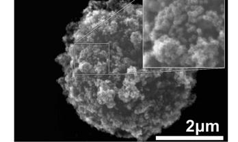
Fig. 1 SEM image of a single magnetic microbead decorated with nanocages. Inset shows a part of the bead imaged at higher magnification. Individual nanocages can clearly be seen on the surface of the microbead
