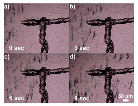
Fig. 5 Magnet-controlled movement of Au nanocages-covered magnetic microbeads towards T-marked area. (a) 1 μl solution of Au nanocages ages-decorated microbeads is dropped away from the marker. Next, the external magnet is placed approximately 1 cm away from the sample. (b)-(d) Gradual movement of the magnetic beads into the desired area.
