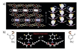
Fig. 9 Two-fold flip-flop motion of m-FAni<sup>+</sup> cations along the C-NH<sub>3</sub><sup>+</sup> axis in monovalent [Ni(dmit)<sub>2</sub>] crystals. (a) Unit cell and supramolecular rotator layer in m-FAni+(dibenzo[18]crown-6)[Ni(dmit)<sub>2</sub>] crystals. (b) The motional freedom of polar m-FAni<sup>+</sup> cations is sensitive to the dielectric response and resulted in the phase transition from the low temperature ferroelectric to the high temperature paraelectric states
