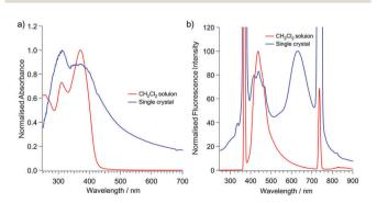
Fig. 3 Absorption (a) and emission (b) spectra of (A)-(+)-1 at room temperature. Red:  $4.0 \times 10^{-5} \; \text{M CH}_2 \text{Cl}_2$  solution. Blue: single crystalline solid.  $\lambda_{ex} = 370 \text{ nm}.$
