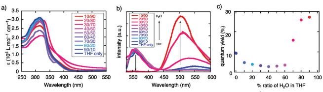
Fig. 2 Photophysical properties of TBFE in a THF/ $H_2O$  mixed solvent system. (a) Absorption spectra (1.0  $\times$  10<sup>-5</sup> M), (b) fluorescence spectra  $(1.0 \times 10^{-6} \text{ M}, \lambda_{\text{ex}} = 317 \text{ nm})$ , and (c) transition of photoluminescence quantum yield measured by the absolute method.
