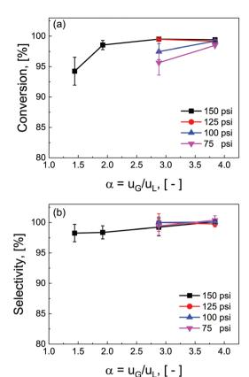
Fig. 3 Multiphase flow optimization. Superficial gas and liquid velocities are screened to achieve maximal (a) conversion, and (b) selectivity at packed bed reactor pressures of 75, 100, 125 and 150 psi. All experiments were conducted at constant liquid flow = 0.4 mL min<sup>-1</sup>. Optimal superficial ratios were at high pressures (150 psi) or large gas flow rates ( $\alpha \ge 1.9$ ).
