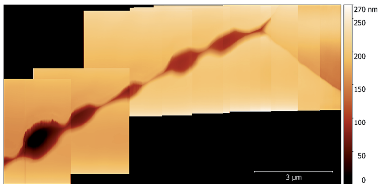
Fig. 6 A topographic map of a number of pits formed along a GB in sensitised AISI 304 stainless steel within 1% aqueous NaCl.
