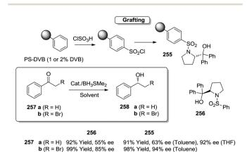
Fig. 64 Polymer supported chiral sulfonamides for the enantioselective reduction of acetophenones.
