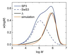
Fig. 9 Comparison of experimentally derived molar mass distributions and a simulated distribution. The label " $\Delta$ " refers to the curve obtained via subtraction of curve SP3 from SwS3. For further details the reader is referred to the main text.
