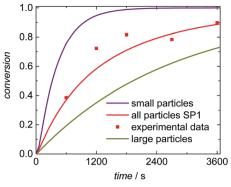
Fig. 7 Simulation results and experimental data of emulsion polymerization SP1. Conversion vs. time data is shown for the total ensemble of particles, for the fraction of small particles with radii between 64.0 and 68.5 nm. and for the fraction of large particles with radii ranging from 118 to 141 nm.
