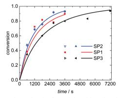
Fig. 6 Conversion vs. time data for seeded emulsion polymerization with identical PSD (SP1 and SP2) or identical  $c_{\rm S}$ (particle) (SP1 and SP3) of the initial seed. The markers represent experimental data and the full lines modeling results. Both SP2 and SP3 refer to two polymerizations carried out at ostensibly identical conditions
