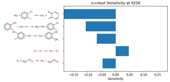
Fig. 9 Sensitivity analysis for OH in the engine-like simulation of 2% mol o-cresol blend in butane given at t = 46.2 ms and T = 925 K. The top 50 sensitive reactions of pure butane were filtered out to underscore the reactions involving o-cresol.
