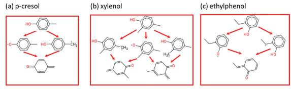
Fig. 11 The P0 reaction pathways of p-cresol, 2.4-xylenol, and xylenol
