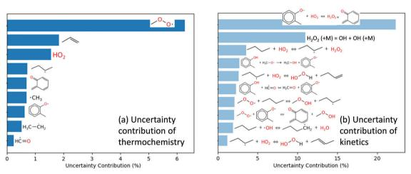
Fig. 10 Local first order uncertainty analysis for OH in the engine-like simulation of 2% mol o-cresol blend in butane given at t = 46.2 ms and T = 925 K.
