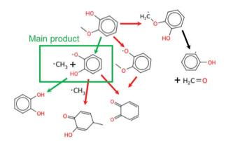
Fig. 12 The main reaction pathways of quaiacol in the engine-like simulation at t = 46.2 ms and T = 925 K.
