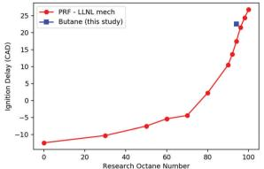
Fig. 2 The computed time of ignition vs. RON for PRFs and n-butane.
