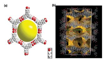
Fig. 1 (a) 2D Hexagonal sheet with a unimodal 3-c hcb (honeycomb) topology in HOF-BTB formed through carboxylic acid dimers. The yellow ball represents a one-dimensional channel with a diameter of ca. 25 nm. (b) Solvent-accessible void space of HOF-BTB calculated with the probe radius of 1.4 Å.
