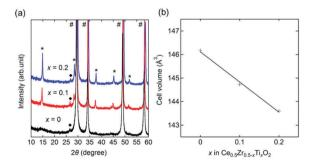
Fig. 1 (a) XRD patterns of  $Ce_{0.5}Zr_{0.5-x}Ti_xO_2$ . Black, red, and blue solid lines represent the patterns of x = 0, 0.1, and 0.2, respectively. Hashtags (#), asterisks (\*), and black squares (\*) indicate peaks arising from the main cubic phase, their superstructure, and unknown impurity, respectively. (b) Cell volumes of  $Ce_{0.5}Zr_{0.5-x}Ti_xO_2$  based on the unit cell of  $Ce_{0.5}Zr_{0.5}O_2$  (Z = 4).
