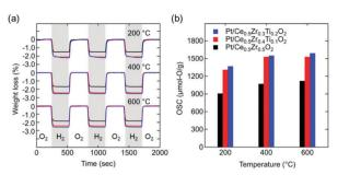
**Fig. 3** (a) TGA curves of Pt/Ce $_{0.5}$ Zr $_{0.5-x}$ Ti $_x$ O $_2$  upon switching between 5% O $_2$ /N $_2$  and 5% H $_2$ /N $_2$  every 5 min at various temperatures. (b) Estimated OSCs. Black, red, and blue lines and columns represent Pt/Ce $_{0.5}$ Zr $_{0.4}$ Ti $_{0.1}$ O $_2$ , and Pt/Ce $_{0.5}$ Zr $_{0.3}$ Ti $_{0.2}$ O $_2$ , respectively.
