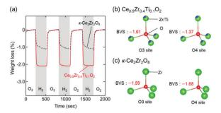
Fig. 5 (a) TGA curves of Pt/Ce<sub>0.5</sub>Zr<sub>0.4</sub>Ti<sub>0.1</sub>O<sub>2</sub> (black dashed line) and  $Pt/\kappa$ - $Ce_2Zr_2O_8$  (red solid line) during the atmosphere switching between  $5\% O_2/N_2$  and  $5\% H_2/N_2$  every 5 min at 200 °C. BVS values of the O3 and O4 sites in (b)  $Ce_{0.5}Zr_{0.4}Ti_{0.1}O_2$  and (c)  $\kappa$ - $Ce_2Zr_2O_8$ .
