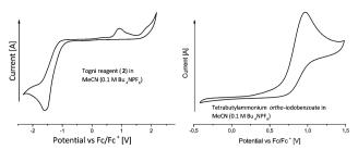
Fig. 2 Cyclic voltammetry of Togni reagent 2 (left) and ortho-iodobenzoate (right).
