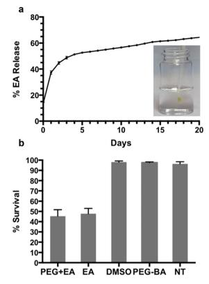
Fig. 4 The release of EA from PEG8H-BA4-EA hydrogel (a); a steady state release of 0.8% per day was observed after day 6. Inset shows a photograph of *in situ* gel formation upon injection of an acidic precursor solution of PEG8H-BA4 and EA into excess buffer at pH 7.4. CAL-27 cell survival rate upon exposure to PEG8H-BA4-EA gel (b). Similar survival rates were observed for both PEG8H-BA4-EA and EA groups, whereas nearly 100% survival was found for the DMSO, PEG8H-BA4, and untreated (NT) groups.
