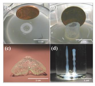
**Fig. 7** Robotic and manual printing of 3D constructs by using an agarose bioink under fluorocarbon. (a) Top and (b) side view of printed cell-laden constructs. (c) 3D construct mimicking a vascular bifurcation that was printed while submerged in perfluorotributylamine. (d) Printed cylinders without cells. <sup>92</sup> Reprinted with permission Copyright IOP Publishing, 2013.
