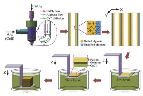
Fig. 4 Bioprinting process of a 3D structure with built-in microchannels by using an alginate bioink. Physical cross-linking process was utilized via calcium ions. 61 Reprinted with permission Copyright Elsevier, 2015.
