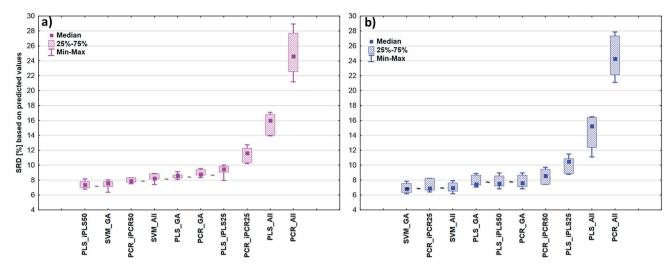
Fig. 4 Box and whisker plots of the transmission spectral models based on SRD in the case of (a) fat content and (b) dry material content. The  $\sim$  mark means that there is no statistically significant difference between the two models according to Wilcoxon's matched pair test at the 5% level.
