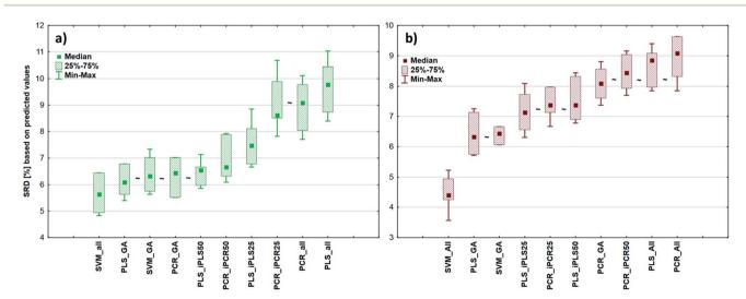
Fig. 5 Box and whisker plots of the reflectance spectral models based on SRD in the case of (a) fat content and (b) dry material content. The  $\sim$  mark means that there is no statistically significant difference between the two models according to Wilcoxon's matched pair test at the 5% level. SRD values based on predicted values were plotted in both cases in %.
