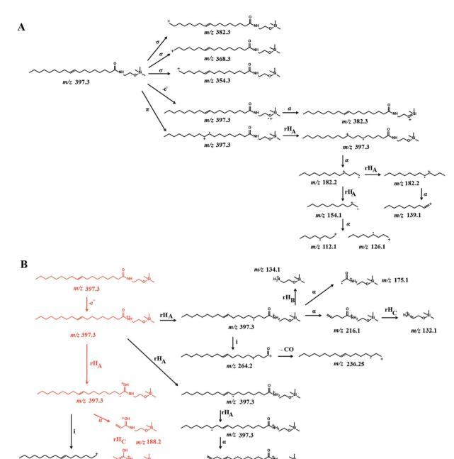
Fig. 2 Proposed EI-CID fragmentation mechanism of OEA: OEA exhibits a molecular ion at m/z 397.3, which undergoes (A) sigma and pi cleavage and (B) hydrogen elimination at different positions, leading to the formation of small fragments at m/z 131.2, 188.2 and are indicated in red. See text for further structural details.
