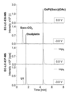
Fig. 4 Chromatographic separation of OxPt(Succ)(OAc) and its respective reduction products obtained by electrochemical conversion at a constant potential of -3.0 V vs. Pd/H<sub>2</sub>. Detection was performed using ESI-MS and complementary ICP-MS.
