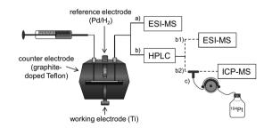
Fig. 1 Instrumental setup for the electrochemical reduction of Pt(v) compounds. (a) Species identification by EC-ESI-MS; (b1) EC-LC-ESI-MS or (b2) EC-LC-ICP-MS analysis of Pt(v) compounds; (c) post-column isotopic dilution analysis for the quantification of Pt species.
