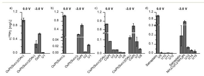
Fig. 5 Quantification results for the different Pt species with (-3.0 V) and without (0.0 V) EC reduction based on a post-column isotopic dilution analysis.
