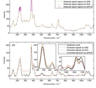
Fig. 10 Real fluorliddicoatite spectrum: (a) signal region detection and (b) signal extraction
