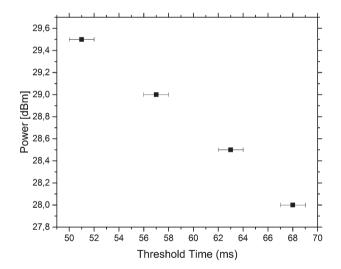
Fig. 5 Power and threshold pulse length needed to push out a droplet. The third trap, being the middle trap, was monitored to measure the minimum time needed to push out a trapped droplet. The threshold time needed to push out increased with the decreasing power of the SAW.
