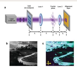
Fig. 1 (a) Projection lithography setup. The addressable SLM is imaged onto a photoalignment surface with magnification factor  $f_2/f_1$ . The amplitude mask in the Fourier plane eliminates unwanted higher diffraction orders. (b) Grayscale input to SLM. Image: Ansel Adams, "The Tetons and the Snake River." (c) Resulting pattern in 1 cm<sup>2</sup> area of a liquid crystal cell, viewed through crossed polarizers (15 µm cell thickness, filled with RM82).
