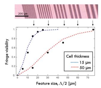
Fig. 4 Fringe visibility of a binary grating as a function of grating pitch. As predicted by a simple model (dashed lines) the measured fringe visibility (solid points) drops as the pitch approaches cell thickness. Two cases are shown: a 15 μm thick cell with 5 μm pixel spacing; and a 50 μm thick cell with 16 µm pixel spacing.
