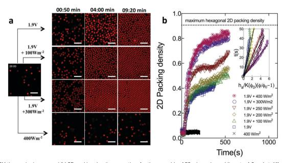
Fig. 1 (a) CLSM time series images and (b) 2D packing density versus time for the assembly of PS microspheres (diameter 1.0 µm) at different conditions of applied electric field voltage and UV power conditions. (inset) Analysis of early assembly time (s) versus  $h_a/K(\Phi_0)(\Phi/\Phi_0-1)$  (m) to determine the deposition Peclet number (Pet). Scale bars are 5 µm.
