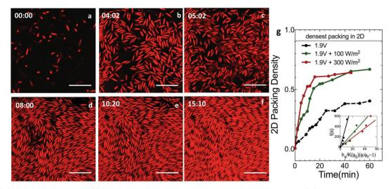
Fig. 2 (a-f) CLSM time series images and (g) 2D packing density versus time for the assembly of PS ellipsoids. CLSM images were taken at the cover slip for self-assembly at 1.9 V and 300 W m<sup>-2</sup> UV illumination. (inset) Analysis of early assembly time (s)  $versus\ h_a/K(\Phi_0)(\Phi/\Phi_0-1)$  (m) to determine the rotational deposition Peclet number (Pe<sub>r</sub>) for the ellipsoid assembly. Scale bars are 10 µm and time stamps are in minutes.
