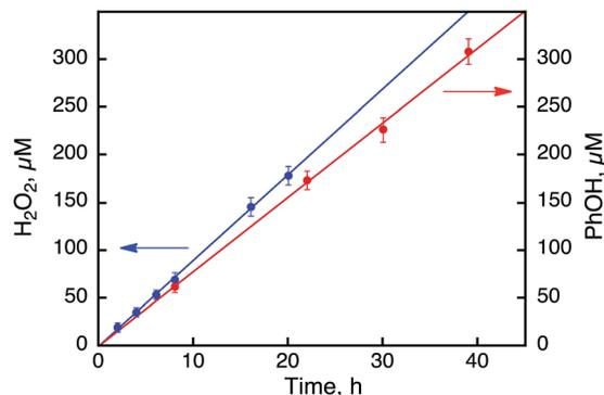
Fig. 7 Time courses of the products from the photoinduced reaction under photoirradiation (white light) in an  $\text{O}_2$ -saturated solvent mixture of MeCN and  $\text{H}_2\text{O}$  ( $v/v = 23 : 2$ ) containing **1** (0.50 mM),  $[\text{Ru}^{\text{II}}(\text{Me}_2\text{phen})_3]^{2+}$  (0.10 mM), and  $\text{Sc}(\text{NO}_3)_3$  (100 mM) in the absence (blue) and presence (red) of benzene (1.0 M) at 298 K.
