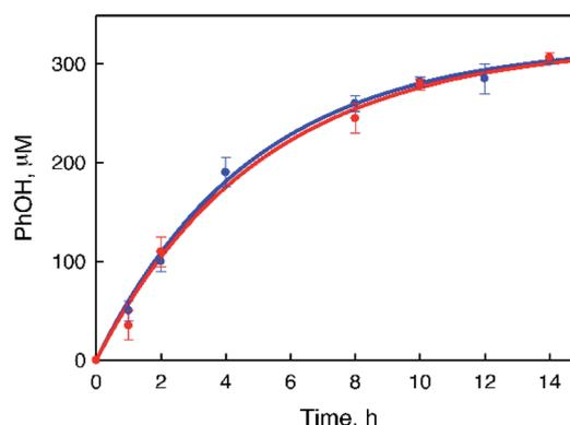
Fig. 2 Time courses of PhOH concentration produced in the photocatalytic oxidation of benzene under photoirradiation (white light) of an  $O_2$ -saturated solvent mixture of MeCN and  $H_2O$  ( $v/v = 23 : 2$ ) containing **1** (0.10 mM),  $[Ru^{II}(Me_2phen)_3]^{2+}$  (1.0 mM), and benzene (1.0 mM, blue circles) or benzene- $d_6$  (1.0 mM, red circles) in the presence of  $Sc(NO_3)_3$  (100 mM) at 298 K. No *p*-benzoquinone was produced under the present experimental conditions.
