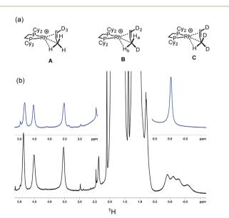
Scheme 9 (a) Isotopomers [1-(d<sub>3</sub>-propene)][BAr<sup>F</sup><sub>4</sub>] highlighting the methyl substitution patterns. (b) <sup>1</sup>H NMR spectra (193 K, CD<sub>2</sub>Cl<sub>2</sub>) of a sample prepared by the solid/gas route after 16 hours. Top,  $[1-(propene)][BAr_4]$ ; bottom,  $[1-(d_3-propene)][BAr_4]$ .
