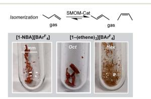
Fig. 8 Representative examples of the physical forms of the various crystalline catalysts used for the gas/solid isomerization of 1-butene to trans and cis-2-butene. SMOM-Cat = solid-state molecular organometallic catalysis.
