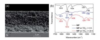
Fig. 2 (a) SEM cross-section image of a Si|mesoTiO<sub>2</sub> electrode. (b) ATR-FTIR spectra of NiP (black), Si|mesoTiO<sub>2</sub>|NiP before (blue) and after (red) 24 h CPP.
